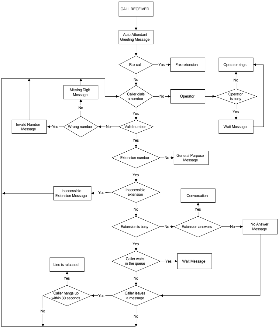
Figure 1- Operation of EVM48 in Day Mode on an Auto Attendant line when Fax Router Mode 1 or Mode 2 is activated as well.
